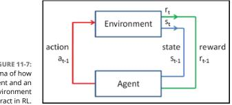
**FIGURE 11-7:** A schema of how an agent and an environment interact in RL.
