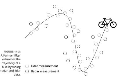
In this way, an SD car can feed the algorithm the sensor measurements and use them to obtain a resulting estimate of the surrounding objects. The estimate combines all the strengths of each sensor and avoids their weaknesses. This is possible because the filter works using a more sophisticated version of probabilities and Bayes' theorem, which are described in Chapter 10.
