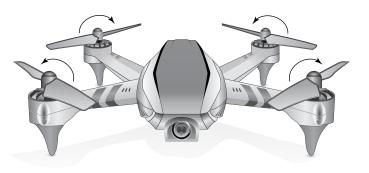
FIGURE 13-1: A quadcopter flies by opportunely spinning its rotors in the right directions.
