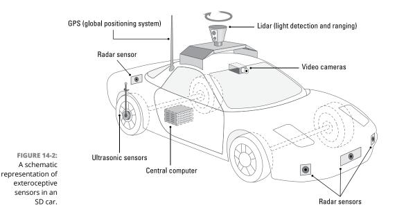
Limitations come in a number of forms. As you explore what sensors do for an SD car, you must consider cost, sensitivity to light, sensitivity to weather, noisy recording (which means that sensitivity of the sensor changes, affecting accuracy), range, and resolution. On the other hand, capabilities involve the capability to track the velocity, position, height, and distance of objects accurately, as well as the skill to detect what those objects are and how to classify them.
