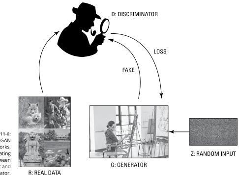
FIGURE 11-6: How a GAN network works, oscillating between generator and discriminator.
